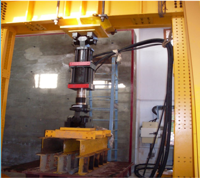
MTS Hydraulic Actuator with Test Frames
