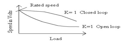
Fig. 6 Speed Vs Load characteristics
