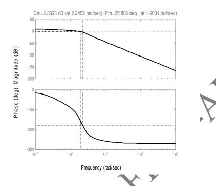
Fig.3 Bode Plot of the System as in Example (3)
