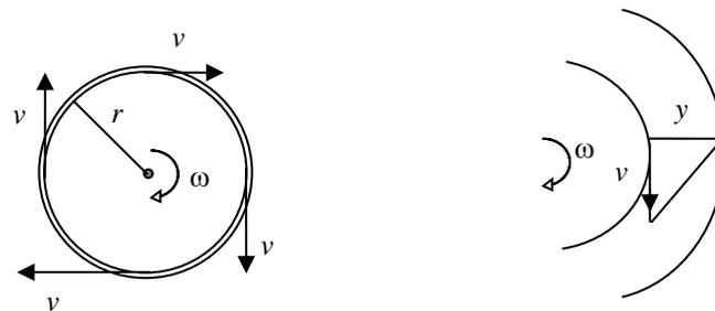
**Figure: Plan view of shaft rotating inside a concentric bearing**
