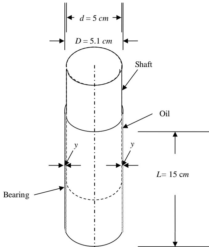
**Figure: Shaft rotating inside a concentric bearing**
