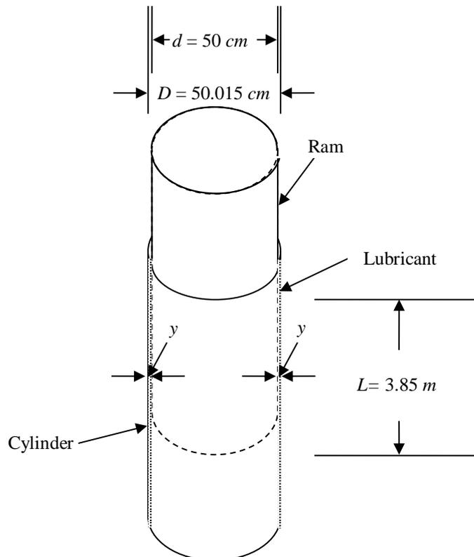
**Figure: Hydraulic Lift with ram and cylinder**
