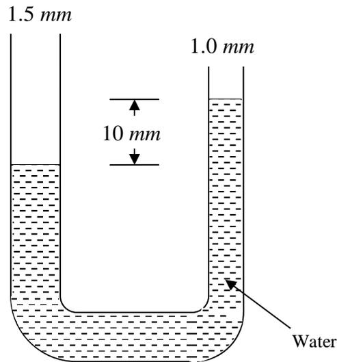
**Figure U – tube containing water**
