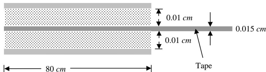
**Figure Tape sliding through the gap filled with lubricant**
