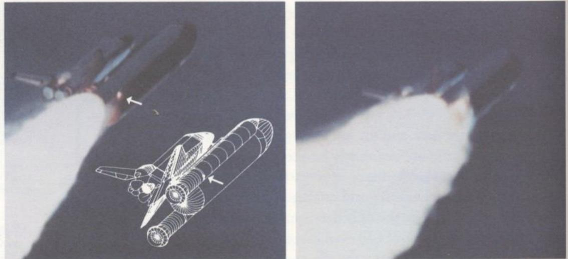
On the launch pad, the leak lasted only about 2 seconds and then apparently was plugged by putty and insulation as the shuttle rose, flying through rather strong cross-winds. Then 58.788 seconds after ignition, when the Challenger was 6 miles up, a flicker of flame emerged from the leaky joint. Within seconds, the flame grew and engulfed the fuel tank (containing liquid hydrogen and liquid oxygen). That tank ruptured and exploded, destroying the shuttle.
