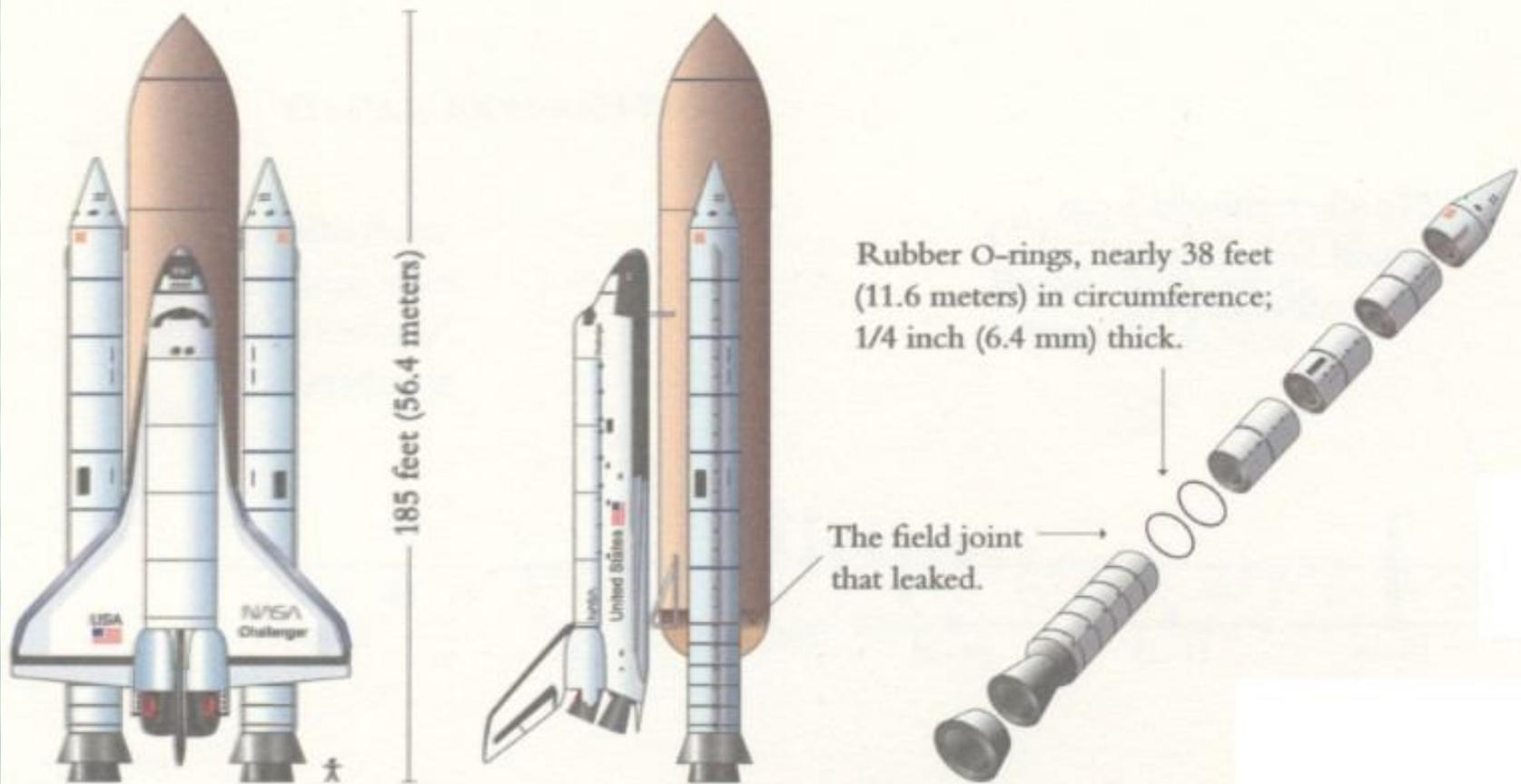
The shuttle consists of an *orbiter* (which carries the crew and has powerful engines in the back), a large liquid-fuel *tank* for the orbiter engines, and 2 solid-fuel *booster rockets* mounted on the sides of the central tank.
