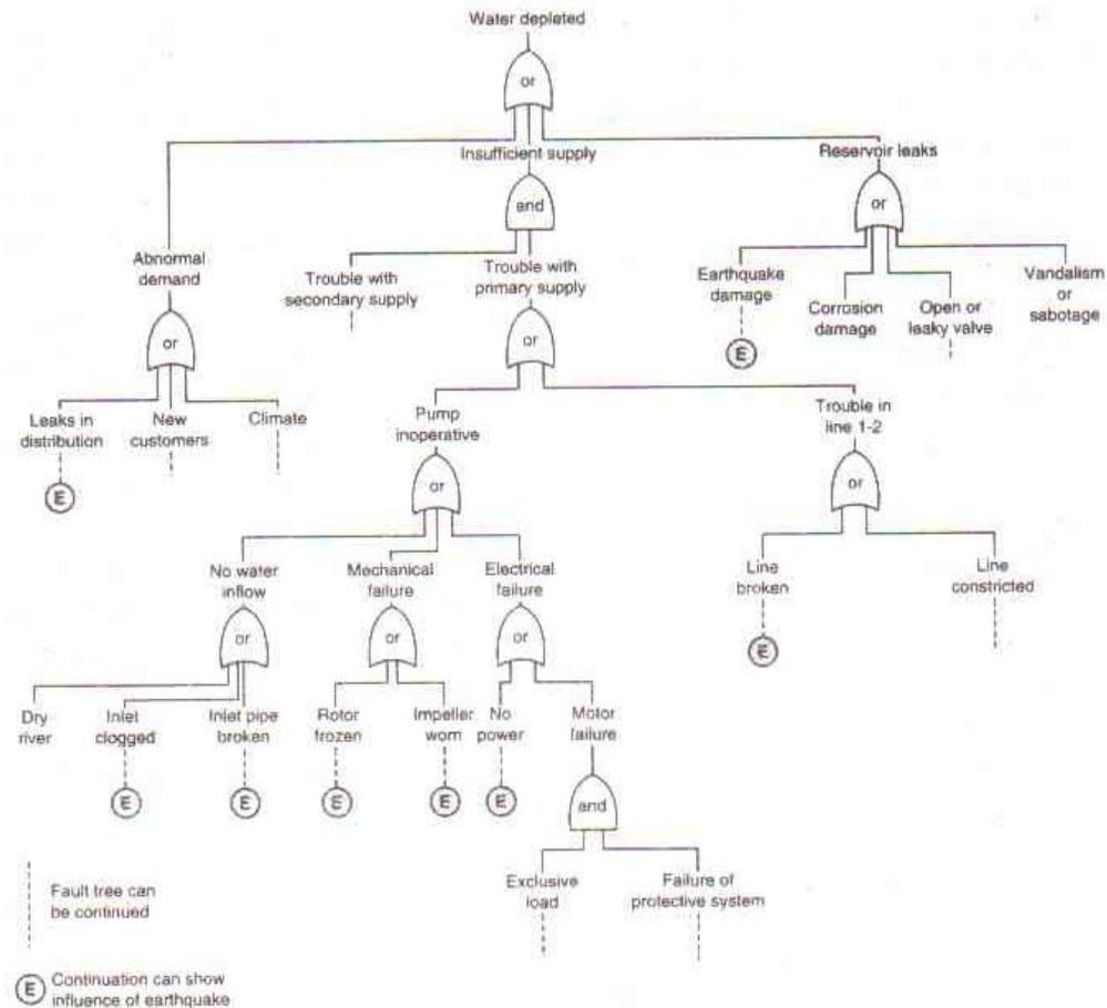
Failure in a Simple Water System analyzed by Fault Tree Analysis
