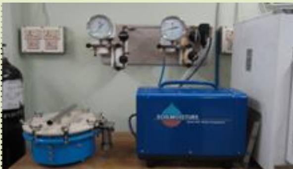
Pressure Plate Apparatus
