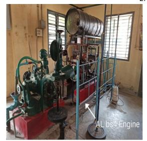
Multi cylinder diesel engine test rig
