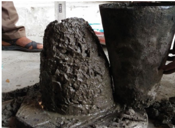
Fig. 4 Slump test on GPC
