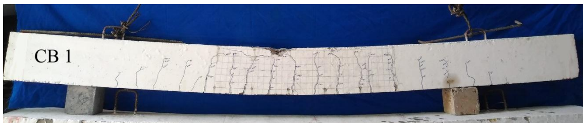
Fig. 6 Crack Pattern of CB1
