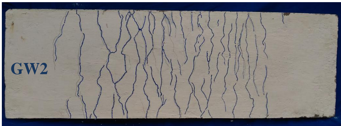
Fig.51 Crack Pattern of (GW2)
