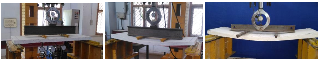
Fig.3(a). Test setup of Slab Panel Fig.3 (b). Deflection of CW1 Fig.3 (c) Deflection of GW1 Slab
