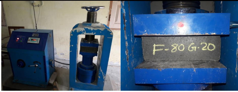
Fig.8 Compressive testing of Geopolymer Brick
