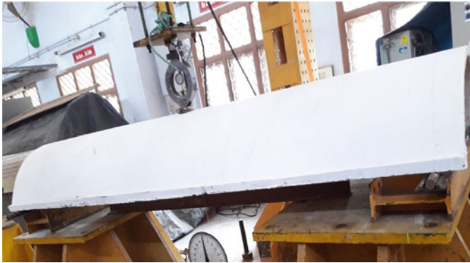
Fig. 22 Test setup of ferrogeopolymer channel
