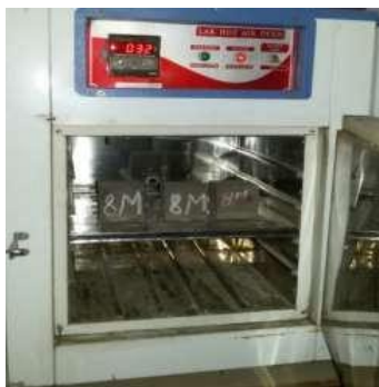
FIG. 4 GEOPOLYMER MORTAR AT OVEN CURING
