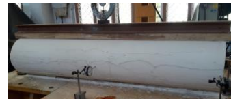
Fig. 16 Test setup of FGPWP
