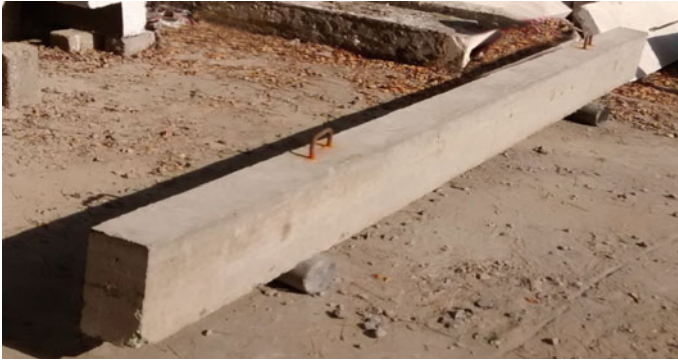
Fig. 9 Ambient curing of geopolymer concrete beam
