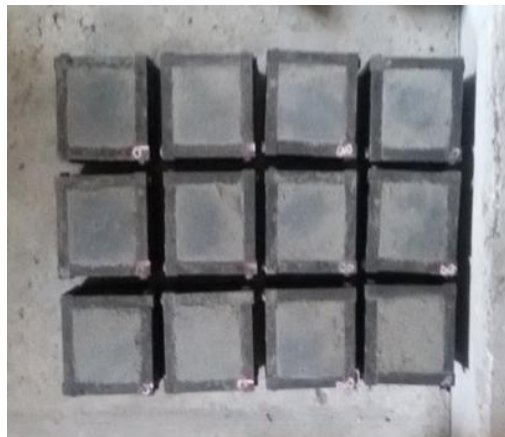
e.Geopolymer Concrete in Moulds
