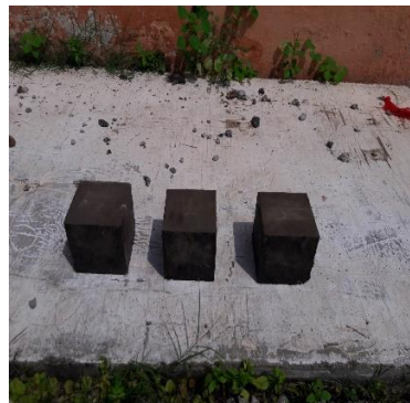
Fig. 2 Curing under Sunlight
