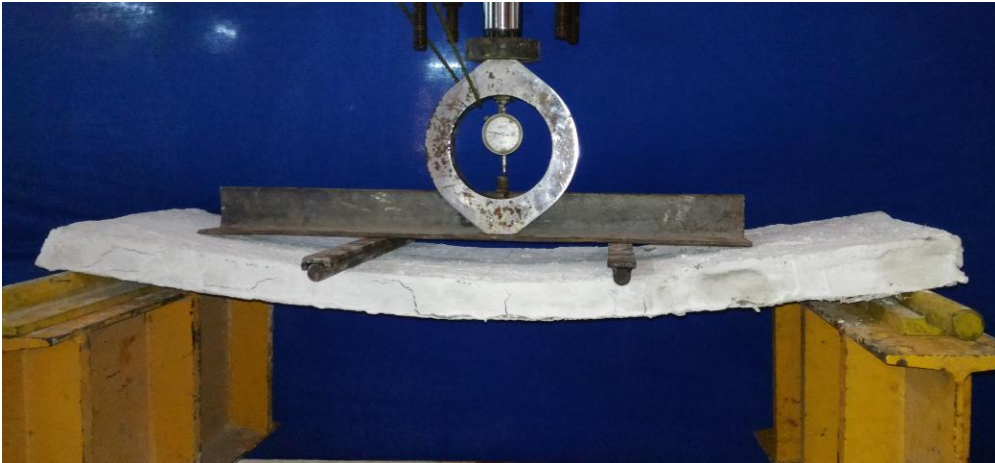
Fig. 46 Deflected Shape @ Ultimate Load (GW1)
