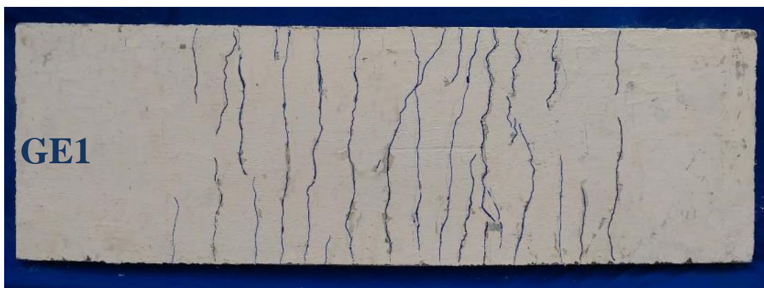
Fig.42 Crack Pattern of (GE1)
