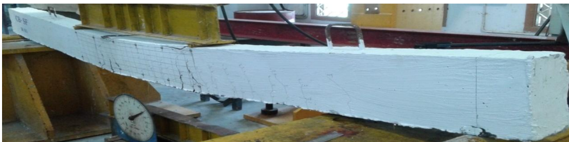
Fig.6 Failure of Beam at Ultimate Load GB1
