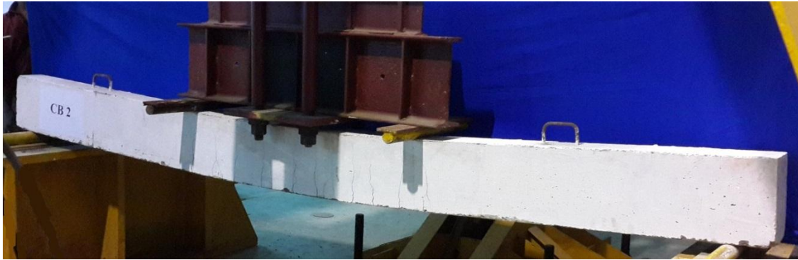
Fig. 10 Failure of Beam at Ultimate Load (CB2)
