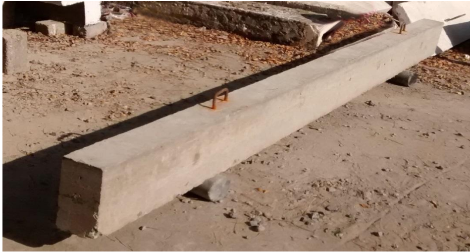
Fig. 3 Ambient curing of Geopolymer Concrete Beam
