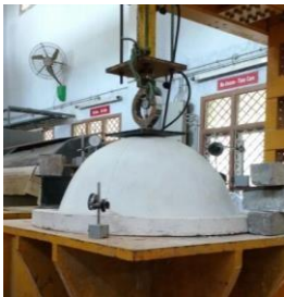
Fig. 10 Test Setup of Dome
