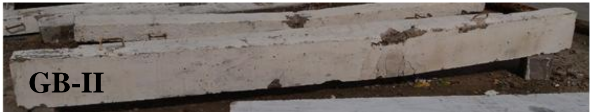
Figure 27 Cracking Pattern of GPC beam Under Cyclic loading
