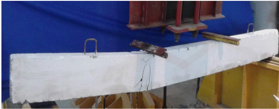
Fig.11 Failure of Beam at Ultimate Load CB2
