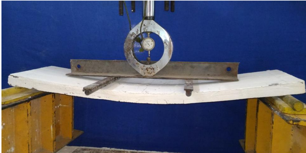
Fig.49 Deflected Shape @ Ultimate Load (GW2)
