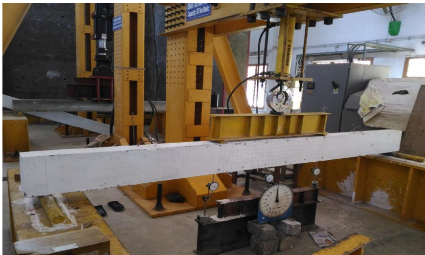
Figure 18 Testing of Beam under Two Point Loading
