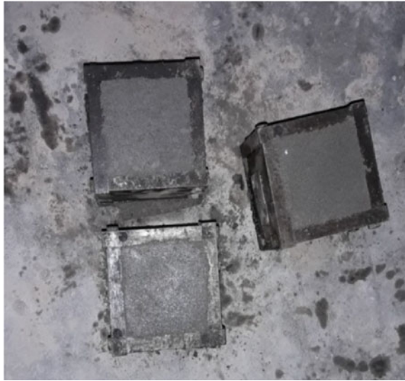
Fig. 5 Casting of GPC cubes
