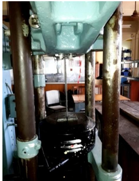
Fig. 2 Tensile Test on Steel Rod
