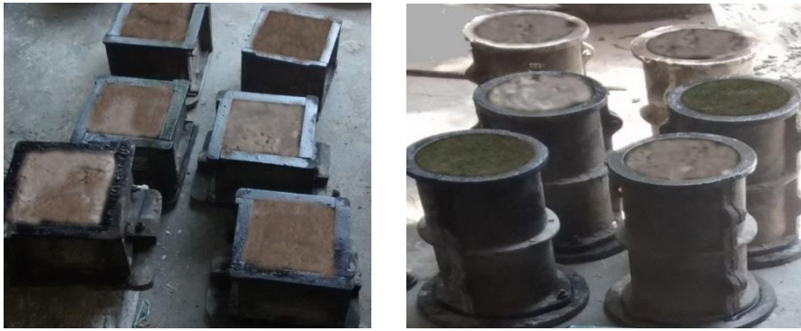
Fig. 2 Casting of Conventional Concrete Cubes and Cylinders
