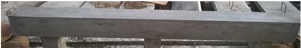
Fig.7 Curing of Ferropolymer Beam (Ambient curing)
