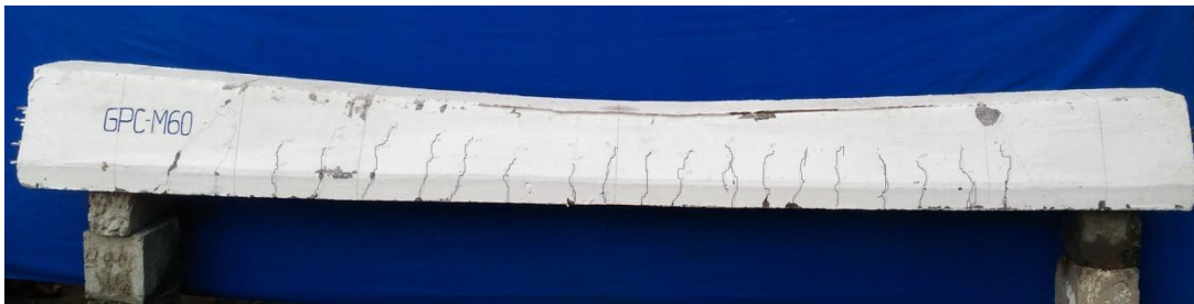
Fig.11 Crack pattern of GPC sleeper
