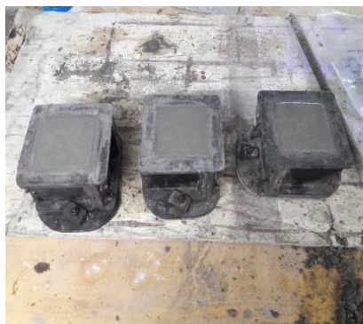
Fig. 1 Casting of Specimen
