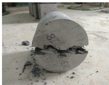
Fig. 5 Cylinder Crack Pattern
