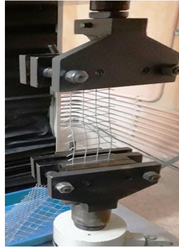
Fig. 4 Test on Welded Wire Mesh
