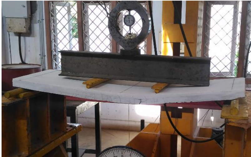
Fig.31 Deflected Shape @ Ultimate Load (CE2)
