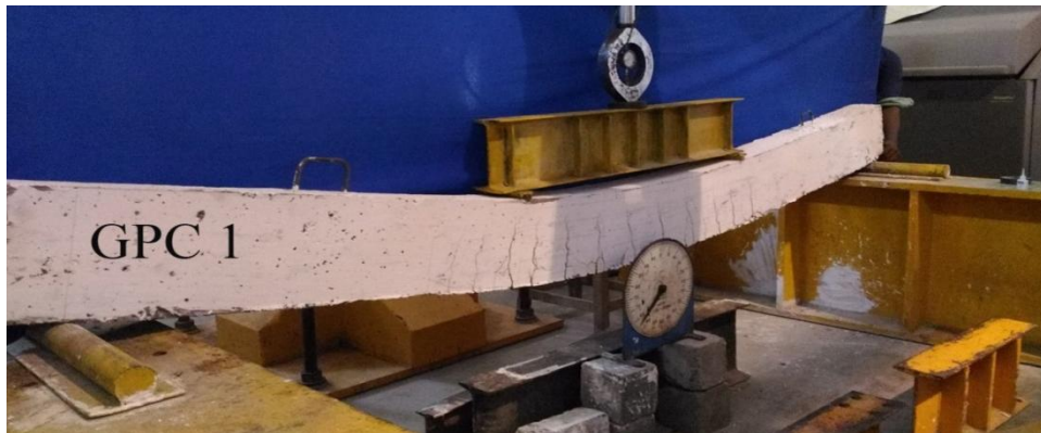
Fig. 5 Failure of Beam at Ultimate Load (GPC1)
