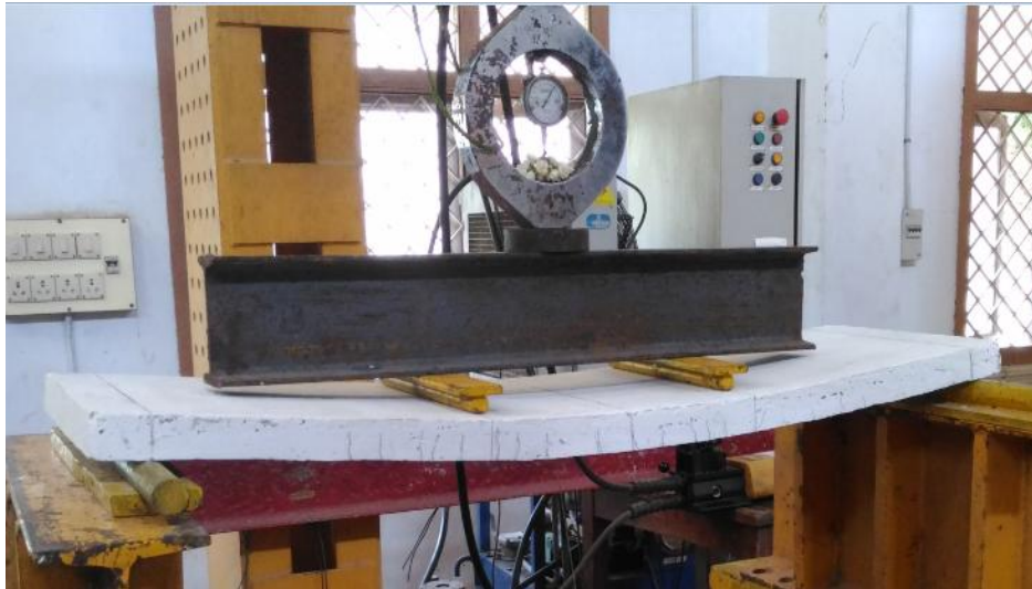
Fig.34 Deflected Shape @ Ultimate Load (CW1)
