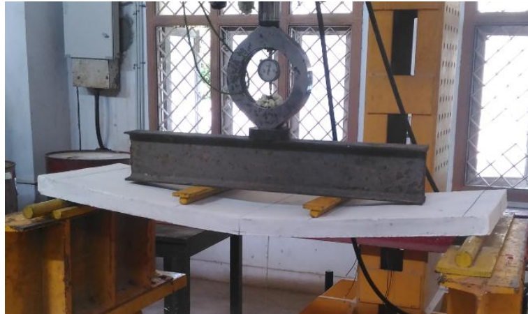
Fig.3.7 Deflected Shape @ Ultimate Load (CW2)
