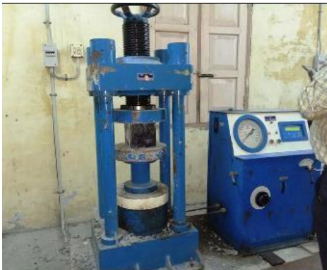
FIGURE 6 COMPRESSION TEST ON CUBE
