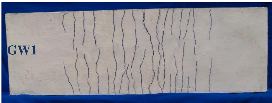
Fig.48 Crack Pattern of (GW1)
