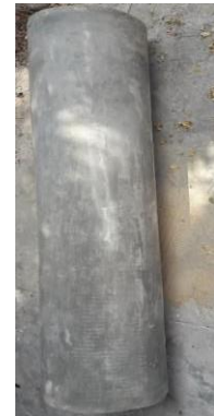
Fig. 15 Casting of Ferro-geopolymer Water Pipes
