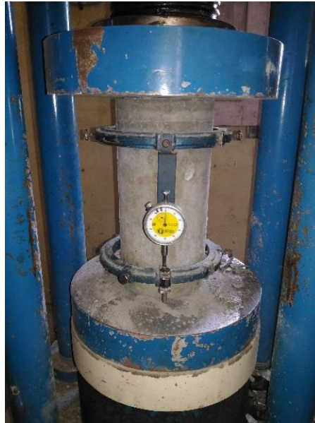
Fig. 8 Test set up for Modulus of Elasticity for Concrete
