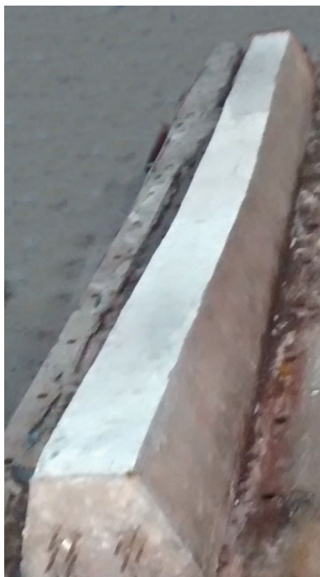
Fig. 18 Ambient curing of GPC sleeper
