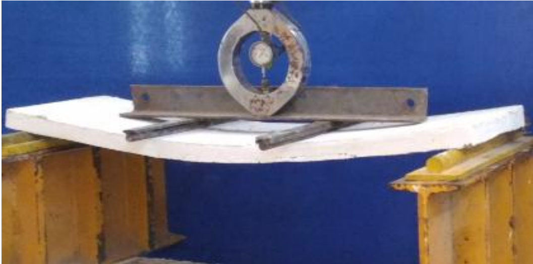
Fig.40 Deflected Shape @ Ultimate Load (GE1)
