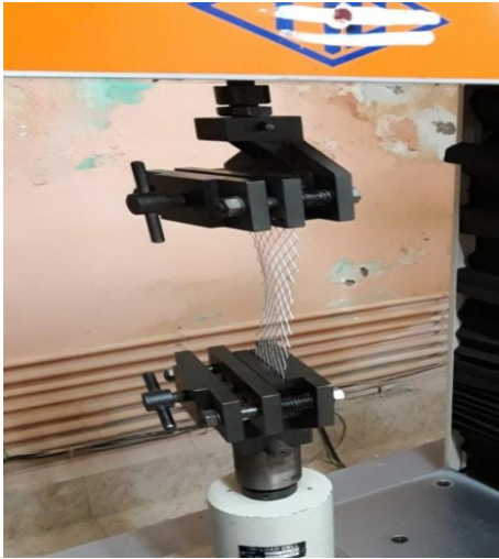
Fig. 3 Test on Expanded Mesh
