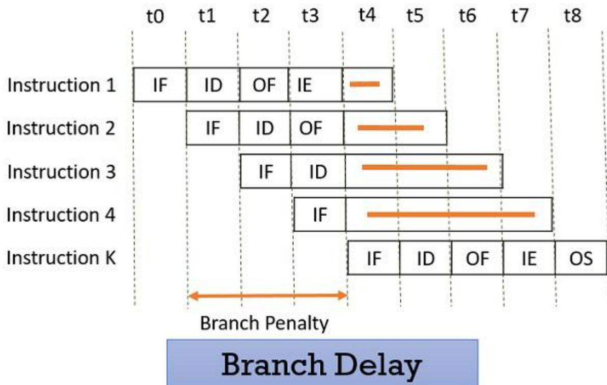
Prefetching the target branch address will reduce the branch delay. Like if the target branch is identified at the decode stage then the branch delay will reduce to 1 clock cycle.
