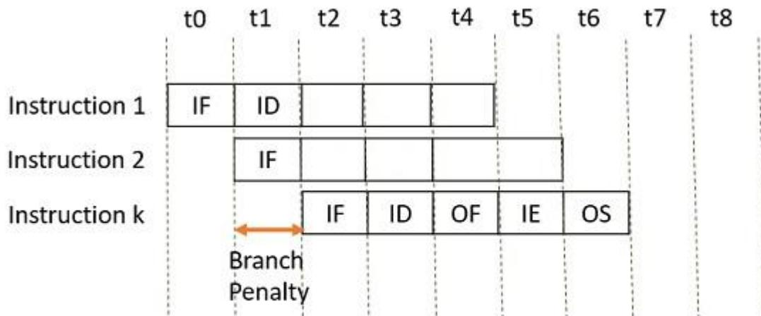
**Branch Delay when Target Branch is Determined at Decode stage**
