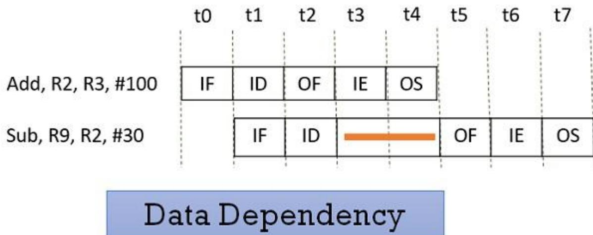
In the figure above, you can see that result of the **Add** instruction is stored in the register **R2** and we know that the final result is stored at the end of the execution of the instruction which will happen at the clock cycle **t4**.
