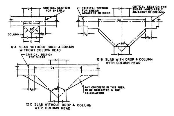
NOTE- D. is the diameter of column or column head to be considered for design.. and d is effective depth of slab or drop
