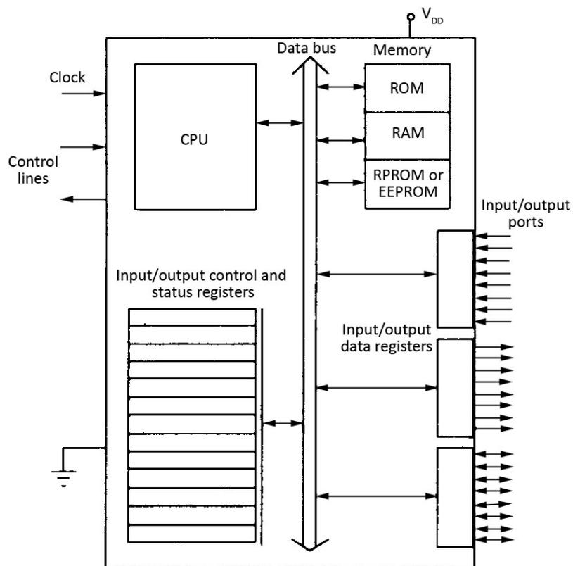
**Figure 28** Block diagram of a microcontroller
