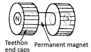
**Figure 15** Hybrid motor rotor
