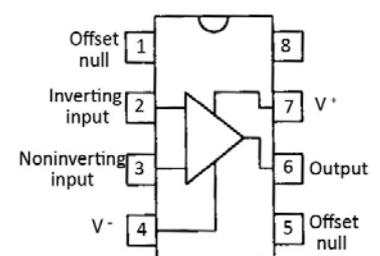
**Figure 30** Pin connections for a
