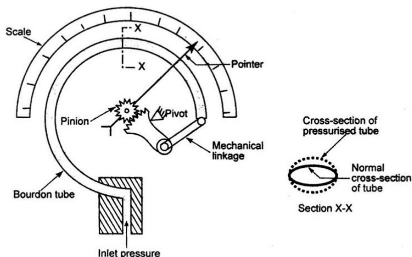
**Figure 16** C-shaped Bourdon tube pressure sensor
