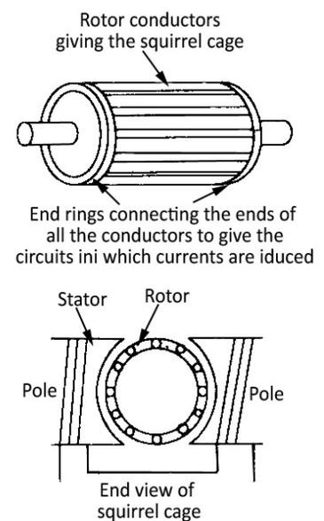
Figure 10 Single-phase induction motor
