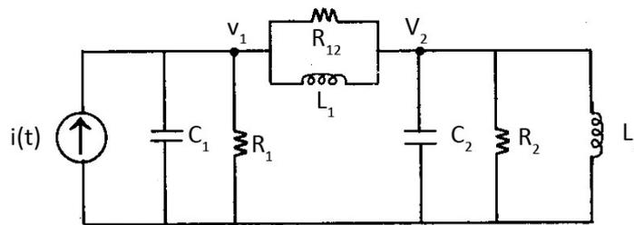
**Figure 7 Force-current electrical analogous circuit**
