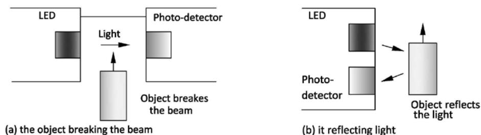
**Figure 24.** Using photoelectric sensor to detect objects
