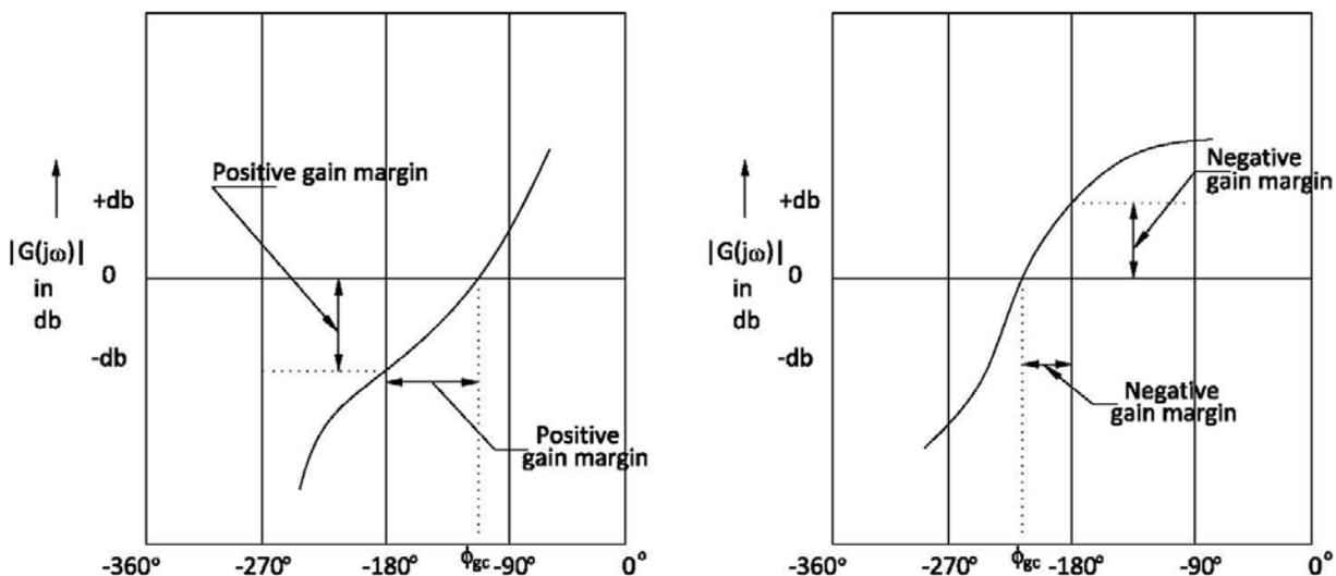
Figure 1 Nichols plot showing phase margin and gain margin
