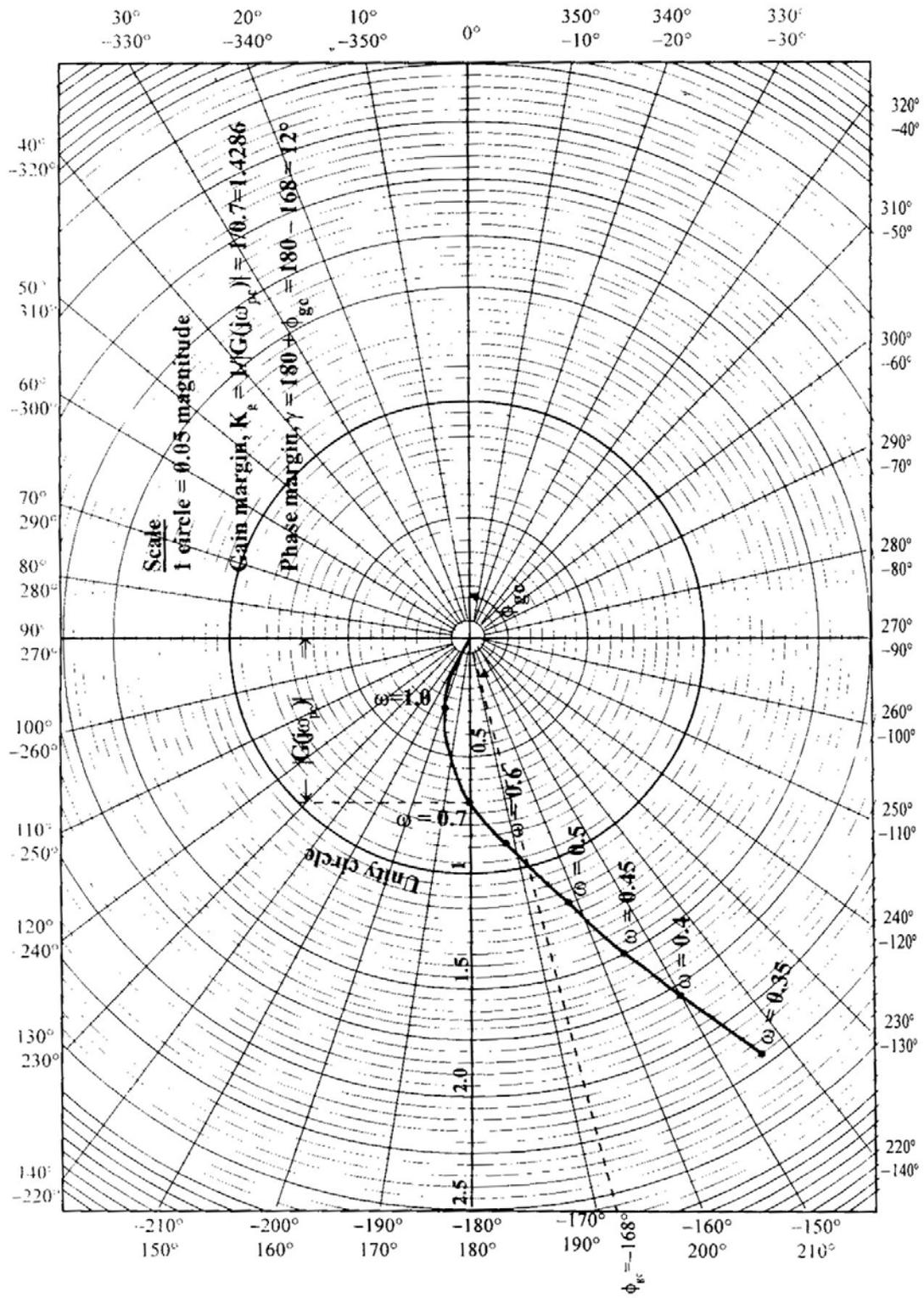
Figure 1 Polar plot of  $G(j\omega) = 1/j\omega(1 + j\omega)$  [using polar coordinates]
