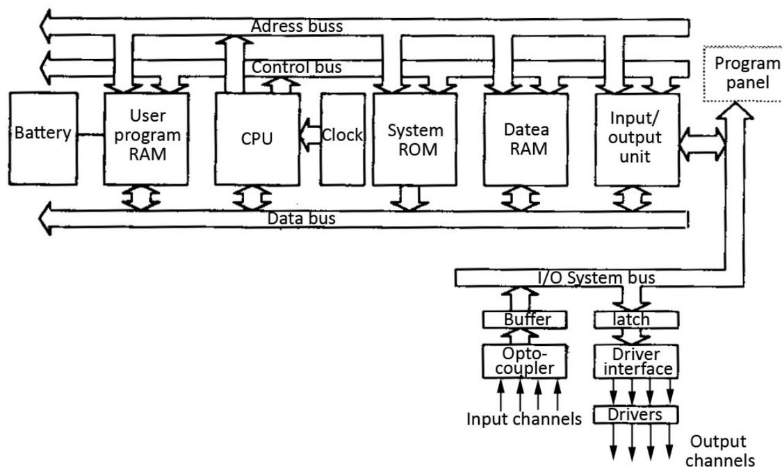
**Figure 4.** Architecture of a PLC
