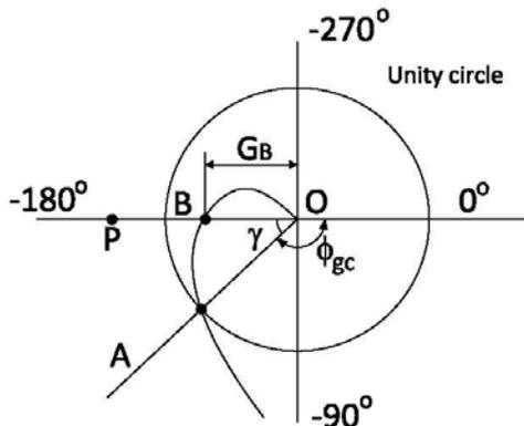
Figure 2.6 Polar plot showing positive gain margin and phase margin.
