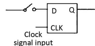
Figure 28. Debouncing a SPDT switch
