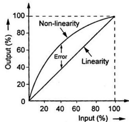
Figure 2 Non-linearity errors
