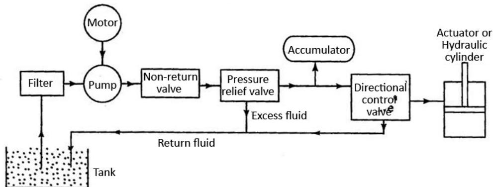
**Figure 18** Basic elements of a hydraulic system
