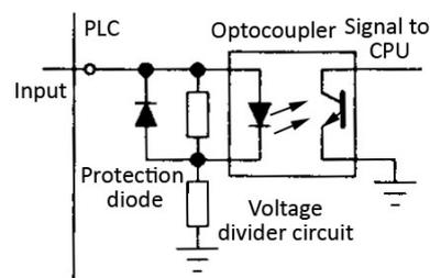
Figure 5. Input channel
