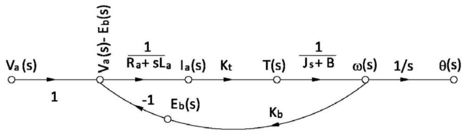
Figure 6 Signal flow graph of armature controlled DC motor
