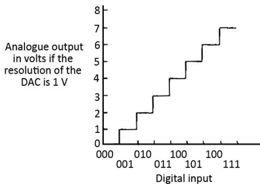
Figure 39 Input-output for a DAC
