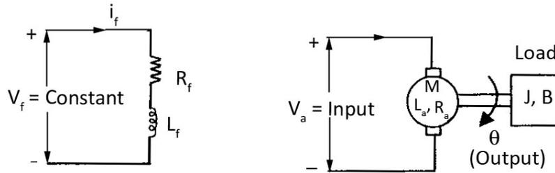
Figure 1.12 Armature controlled DC motor
