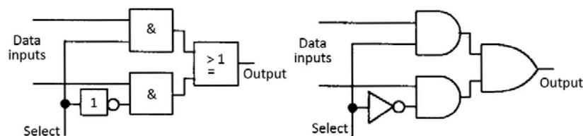
Figure 49 Two channel multiplexer
