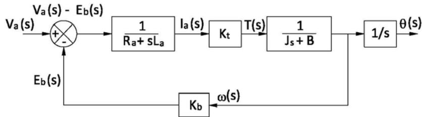
Figure 6 Block diagram of armature controlled dc motor
