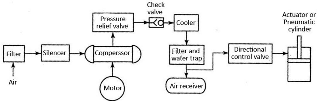
**Figure 17** Basic elements of a pneumatic system
