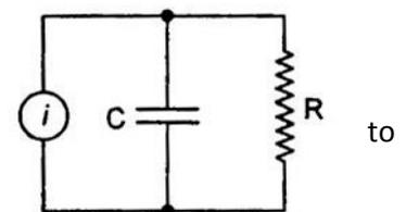
**Figure 8** Equivalent circuit of a pyroelectric sensor
