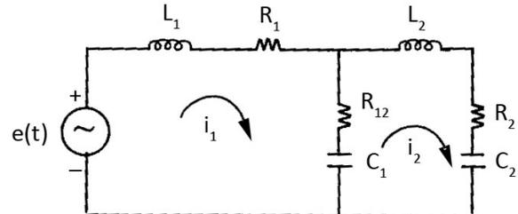
Figure 4 Force-voltage electrical analogous circuit
