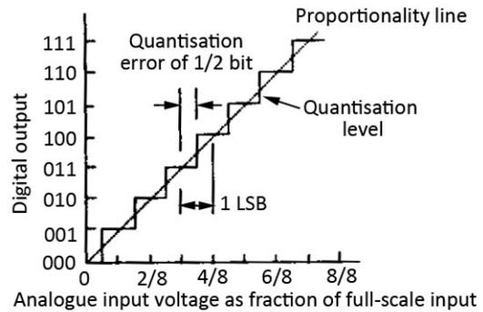
Figure 40 Input-output for an ADC
