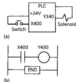
**Figure 7.** Switch controlling a solenoid
