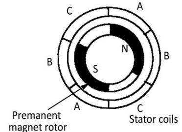
Figure 9 Brushless permanent magnet dc motor
