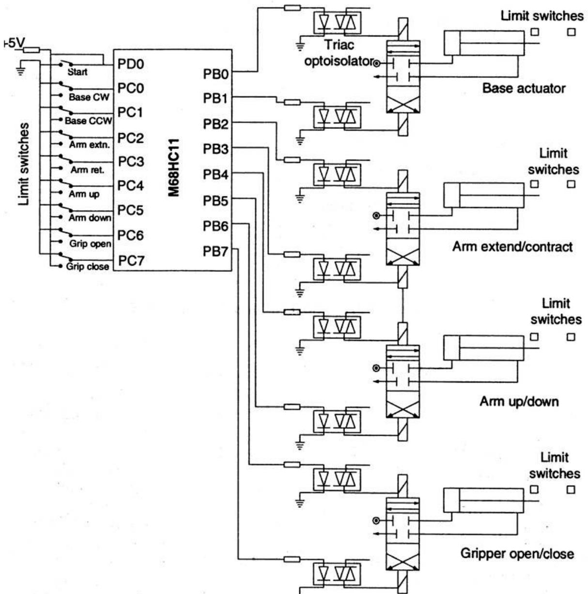
Figure 11 Microcontroller circuit for pick and place robot
