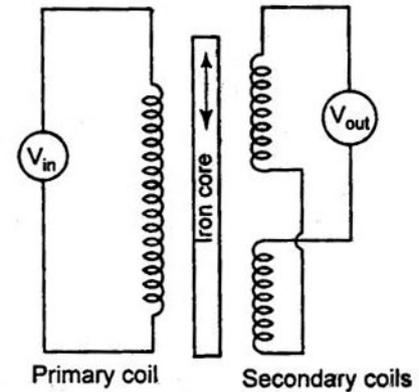
Figure 3 LVDT (Linear variable differential transformer)
