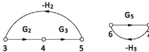
**Figure 8 Second combination of two non touching loops**
