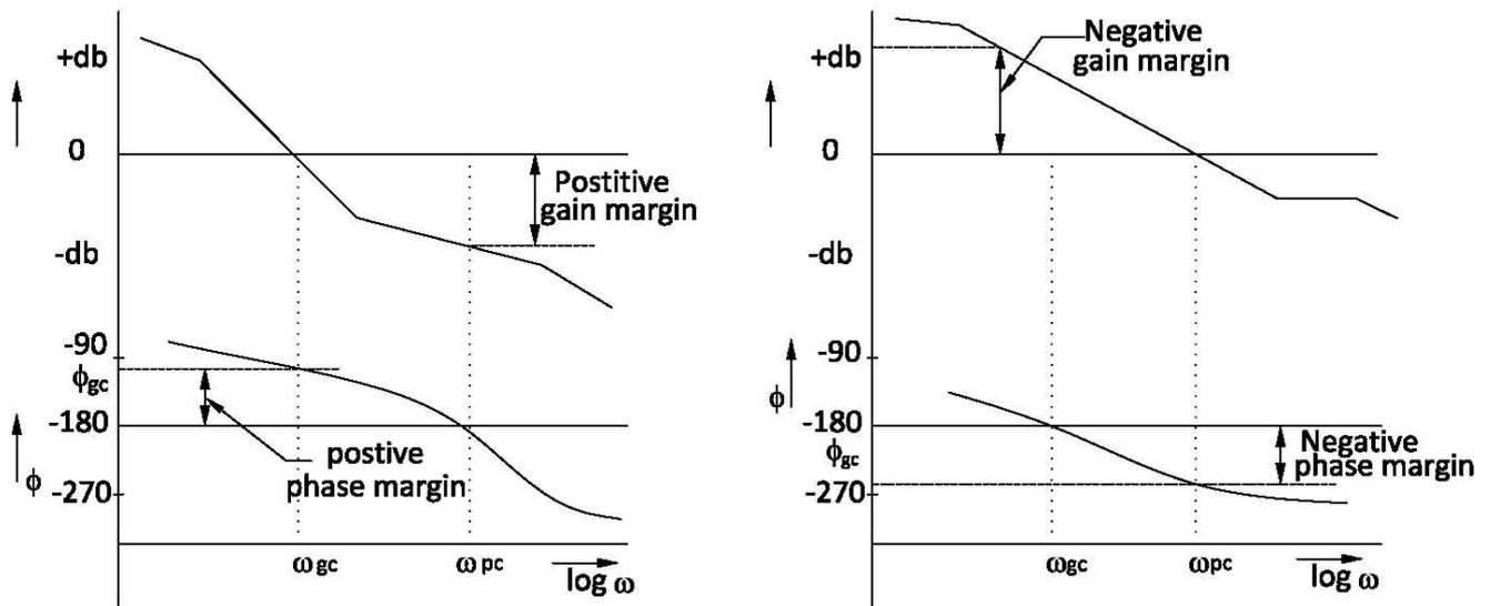
Figure 2.8 Bode plot showing phase margin ( $\gamma$ ) and gain margin ( $K_g$ )
