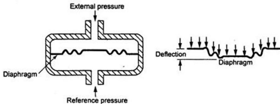
Figure 12 Typical diaphragm pressure gauge
