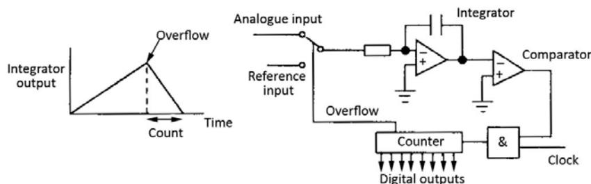
**Figure 46** Dual ramp ADC
