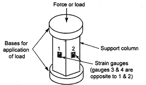
(a) Structure of load cell
