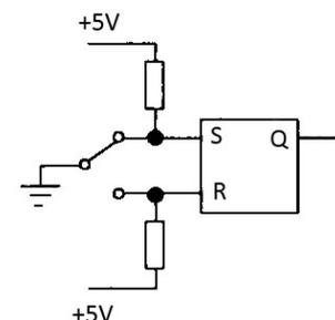
Figure 27 Debouncing a SPDT switch
