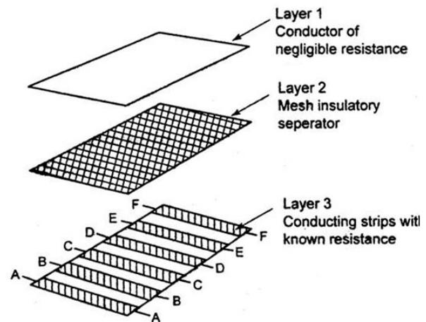
**Figure 20** Tactile pressure sensor
