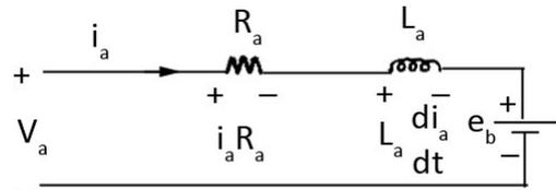
Figure 1.13 Equivalent circuit of armature
