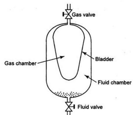
**Figure 19** Hydraulic accumulator
