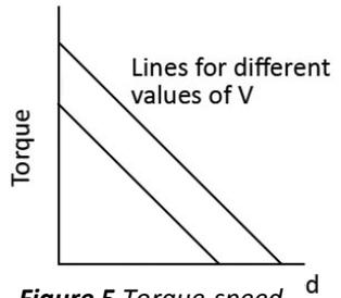
Figure 5 Torque-speed characteristic
