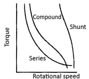
Figure 7 Torque-speed characteristics
