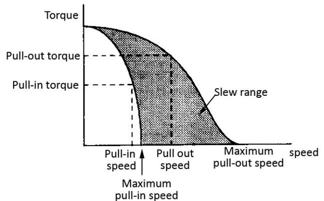
Figure 16 Stepper motor characteristics
