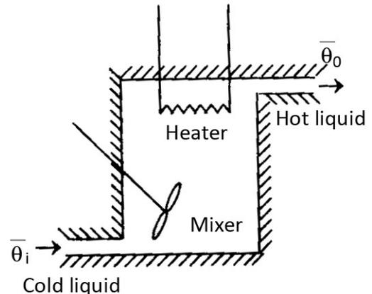
Figure 1.10 Thermal system
