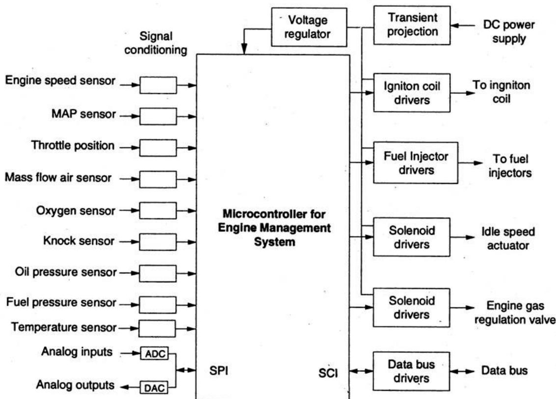
**Figure 14** Interfacing of sensor with controller in engine management system
