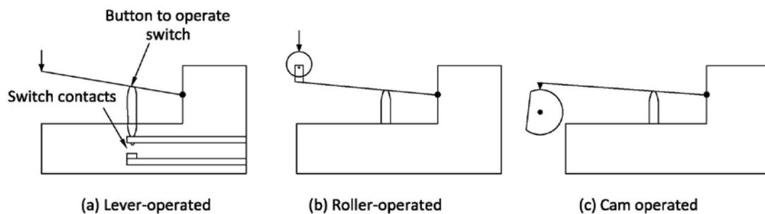
**Figure 22.** Various types of switches
