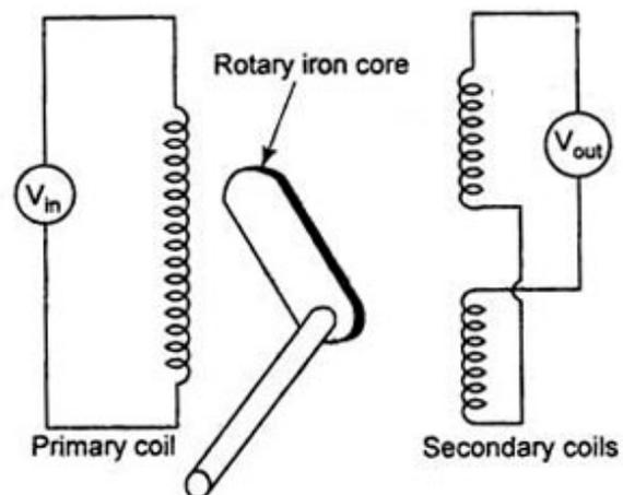
Figure 5 RVDT (Rotary variable differential transformer)
