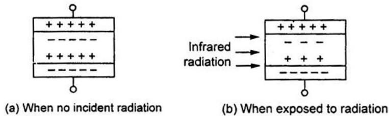
**Figure 7** Pyroelectric effect
