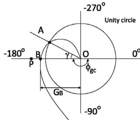
Figure 2.7 Polar plot showing negative gain margin and phase margin.
