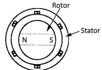
**Figure 12** Three-phase synchronous motor
