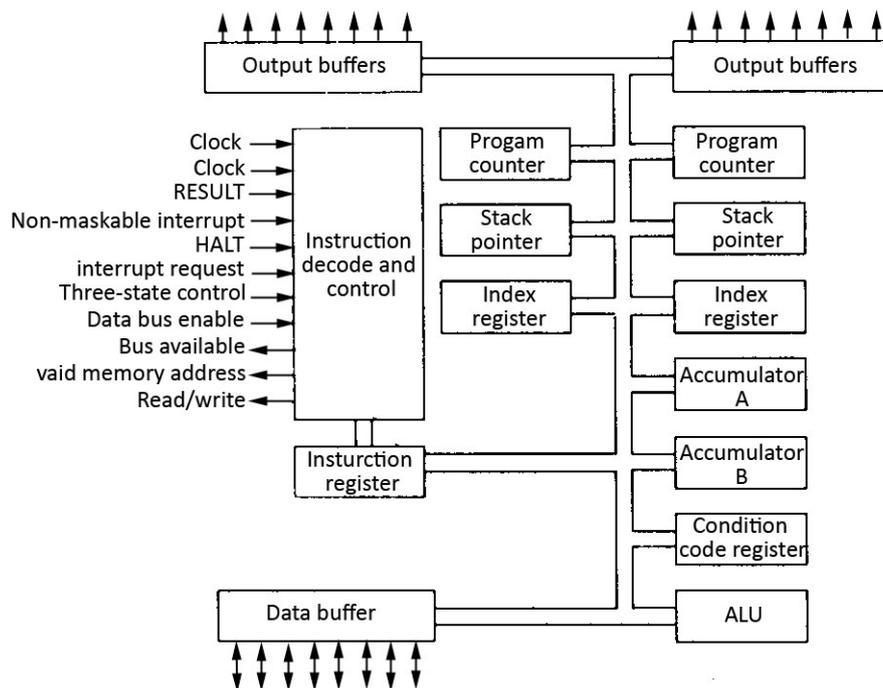
**Figure 23** Motorola 6800 architecture
