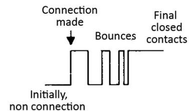
Figure 26 Switch bounce on closing a switch
