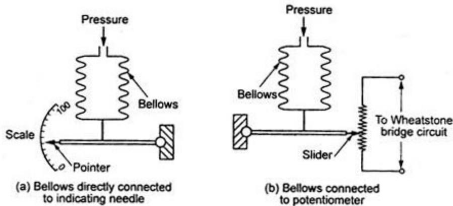
**Figure 15** Bellow pressure sensor
