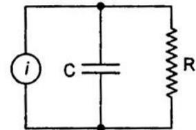
**Figure 19** Equivalent circuit of Piezoelectric sensor
