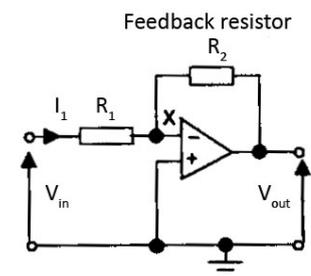
Figure 31 Inverting amplifier
