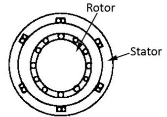
**Figure 11** Three-phase induction motor
