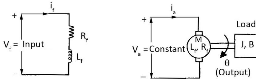
Figure 1.15 Field controlled DC motor
