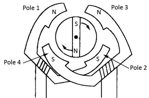
**Figure 14** Permanent magnet stepper motor
