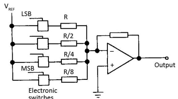
Figure 41 Weighted-resistor DAC
