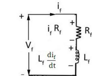
Figure 1.16 Equivalent circuit
