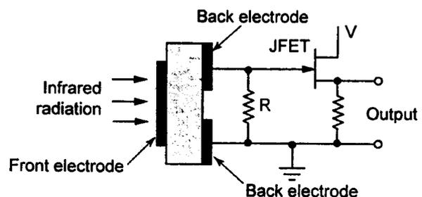
**Figure 9** Dual pyroelectric sensor
