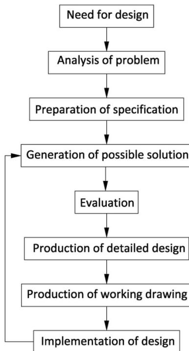
**Figure 8.** Stages in designing mechatronics systems
