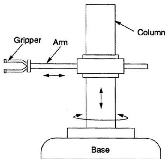
**Figure 9.** Basic form of a pick and place robot
