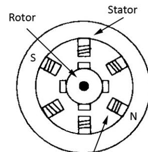
This pair of poles energised by current being switched to them and rotor rotates to position shown below
