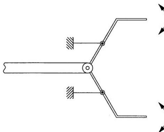
**Figure 10.** Gripper mechanism of a robot
