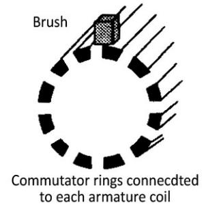
Figure 8 Commutator
