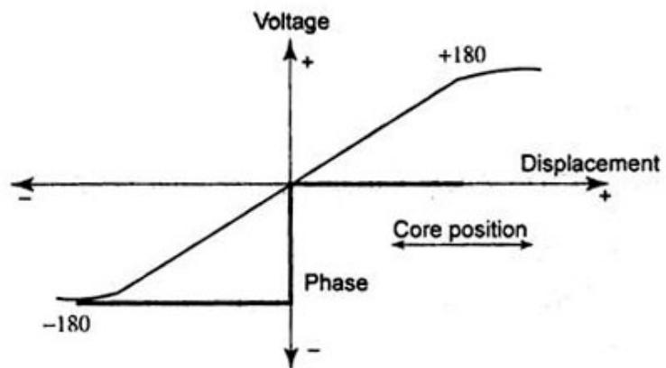
Figure 4 LVDT output
