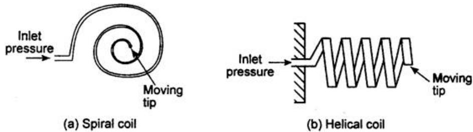
Figure 17 Spiral and helical coil Bourdon tubes
