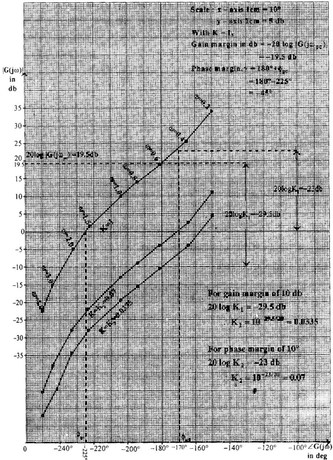
Figure 1 Nichols plot of  $G(j\omega) = \frac{(1+j10\omega)}{(j\omega)^2(1+j\omega)(1+j2\omega)}$
