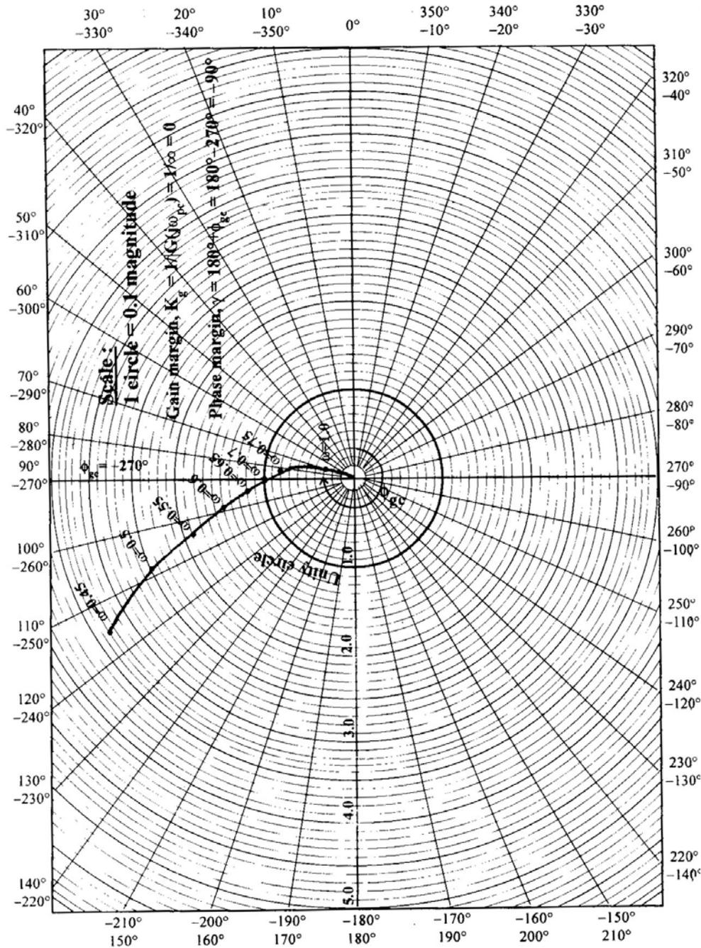
Figure 1 Polar plot of  $G(j\omega) = 1/(j\omega)^2 (1 + j\omega)^2 (1 + j2\omega)$ , Using polar coordinates
