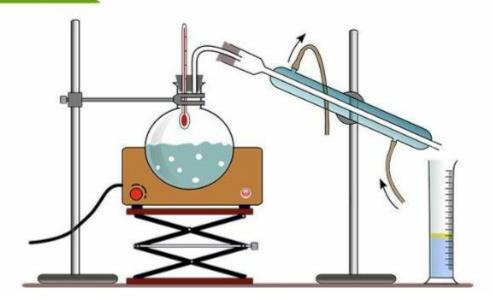
The distillation performed on a laboratory scale often uses batches of the liquid mixture whereas industrial distillation processes are generally continuous, requiring a constant composition of the mixture to be maintained.
