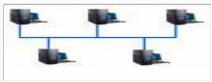
Each host has a unique hardware address. **Packets** are sent out onto the **bus**. The data packet contains the address of the sender and receiver. The receiver will only access the data once the address has been read.
